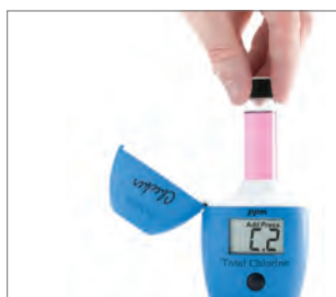
Place the vial into your Checker®HC
